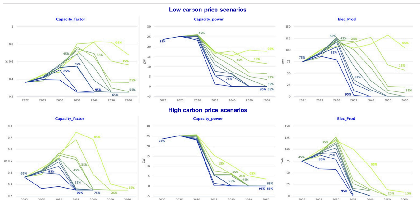
Figure 8. Capacity factor (left panel), capacity (middle), and electricity production (right) for uncontrolled gas combined cycle fleet.
